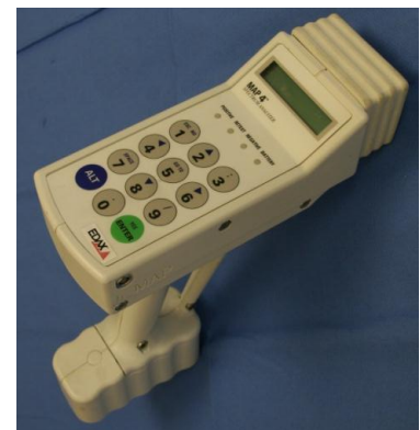
Figure 6: Niton and MAP-4 handheld XRF units, 1994-1995.
