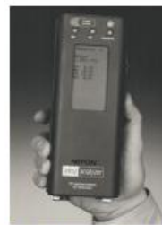
1994: NITON XL-309 1 st one piece, handheld XRF with real-time digital signal processing and silicon PIN diode detectors
