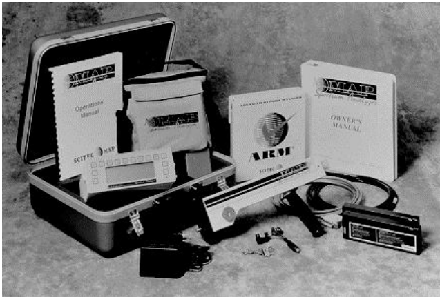
Figure 4: The MAP-3 analyzer in 1997, the beginning of true HH XRF.
