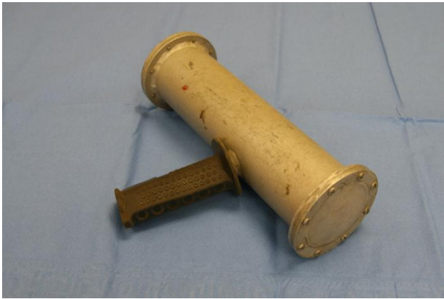
Figure 1: DOE/United Nuclear “hand held” XRF measurement head.
